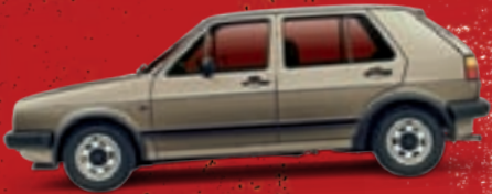
Golf Mk II GTI: The chassis of the GTI was ten millimetres lower than the other models of the second Golf generation.
